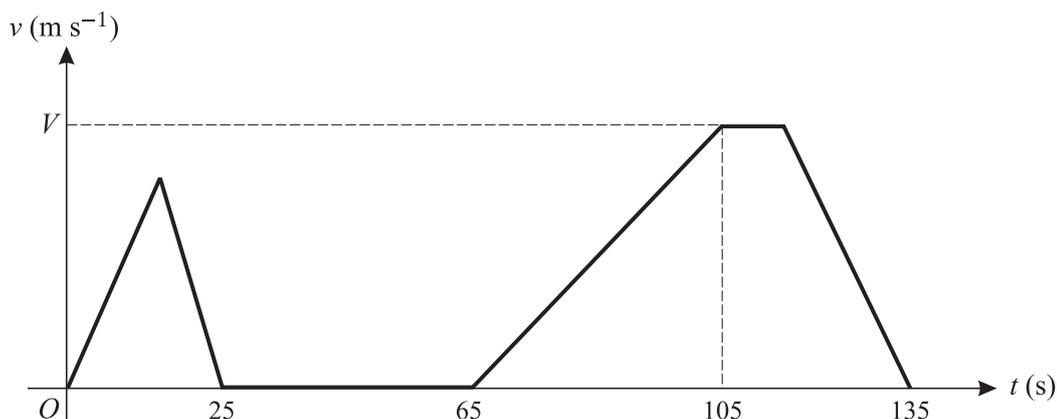
The diagram shows the  $(t, v)$  graph for the motion of a hoist used to deliver materials to different levels at a building site. The hoist moves vertically. The graph consists of straight line segments. In the first stage the hoist travels upwards from ground level for 25 s, coming to rest 8 m above ground level.
