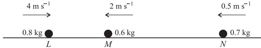
Three uniform spheres  $L$ ,  $M$  and  $N$  have masses  $0.8\text{ kg}$ ,  $0.6\text{ kg}$  and  $0.7\text{ kg}$  respectively. The spheres are moving in a straight line on a smooth horizontal table, with  $M$  between  $L$  and  $N$ . The sphere  $L$  is moving towards  $M$  with speed  $4\text{ m s}^{-1}$  and the spheres  $M$  and  $N$  are moving towards  $L$  with speeds  $2\text{ m s}^{-1}$  and  $0.5\text{ m s}^{-1}$  respectively (see diagram).
