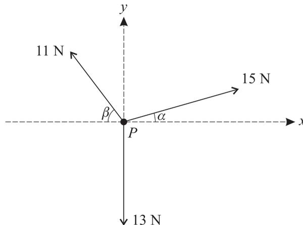
Three horizontal forces of magnitudes 15 N, 11 N and 13 N act on a particle  $P$  in the directions shown in the diagram. The angles  $\alpha$  and  $\beta$  are such that  $\sin \alpha = 0.28$ ,  $\cos \alpha = 0.96$ ,  $\sin \beta = 0.8$  and  $\cos \beta = 0.6$ .
