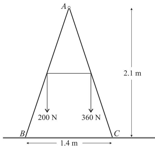
Two uniform rods  $AB$  and  $AC$ , of equal lengths, and of weights  $200 \text{ N}$  and  $360 \text{ N}$  respectively, are freely jointed at  $A$ . The mid-points of the rods are joined by a taut light inextensible string. The rods are in equilibrium in a vertical plane with  $B$  and  $C$  in contact with a smooth horizontal surface. The point  $A$  is  $2.1 \text{ m}$  above the surface and  $BC = 1.4 \text{ m}$  (see diagram).
