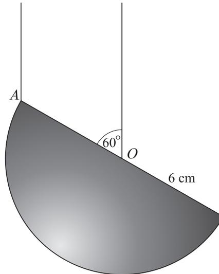
A uniform solid hemisphere of weight 12 N and radius 6 cm is suspended by two vertical strings. One string is attached to the point  $O$ , the centre of the plane face, and the other string is attached to the point  $A$  on the rim of the plane face. The hemisphere hangs in equilibrium and  $OA$  makes an angle of  $60^\circ$  with the vertical (see diagram).
