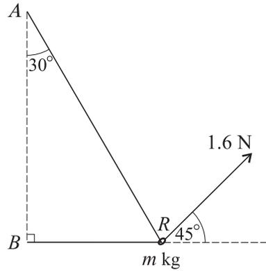
A light inextensible string has its ends attached to two fixed points  $A$  and  $B$ . The point  $A$  is vertically above  $B$ . A smooth ring  $R$  of mass  $m$  kg is threaded on the string and is pulled by a force of magnitude  $1.6$  N acting upwards at  $45^\circ$  to the horizontal. The section  $AR$  of the string makes an angle of  $30^\circ$  with the downward vertical and the section  $BR$  is horizontal (see diagram). The ring is in equilibrium with the string taut.
