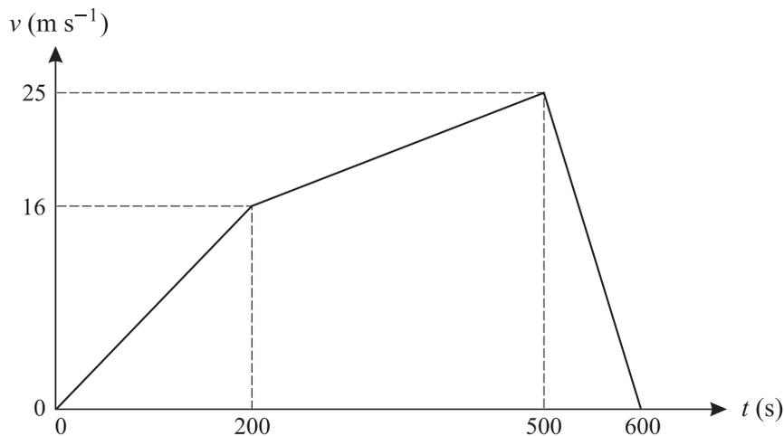
A car  $P$  starts from rest and travels along a straight road for  $600 \text{ s}$ . The  $(t, v)$  graph for the journey is shown in the diagram. This graph consists of three straight line segments. Find
